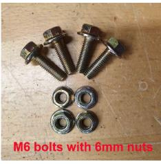
**Step 1**. Place the seat/backrest assembly upside down on a table or chair. Remove the 4 x M6 bolts so that the 4-legged frame can be attached to the swivel mechanism. It is easier if the swivel mechanism is rotated as shown above so that the 4 fixing holes in the swivel mechanism are "exposed".
